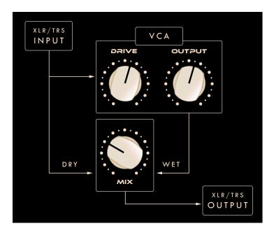
On the Mix control, counterclockwise is your Dry signal, at unity gain, straight off the Inputs, untouched by any further circuitry. Clockwise is the signal post-VCA, and therefore post-saturation/distortion/compression.
