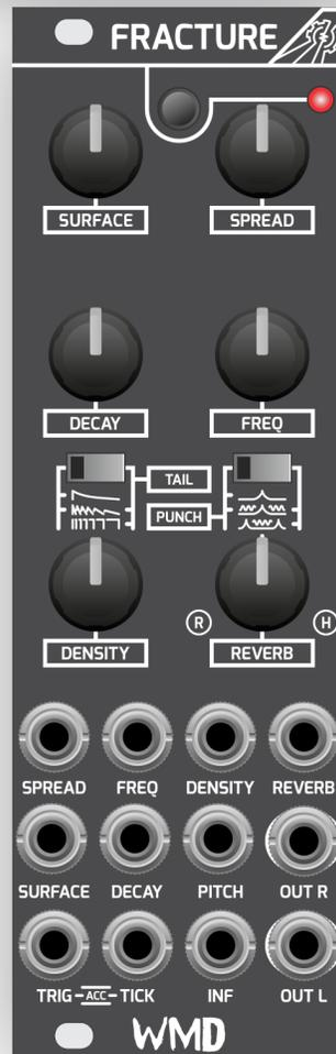
**SPREAD:** As SPREAD is increased the particles are assigned pitches and panning with greater variance from the center.
