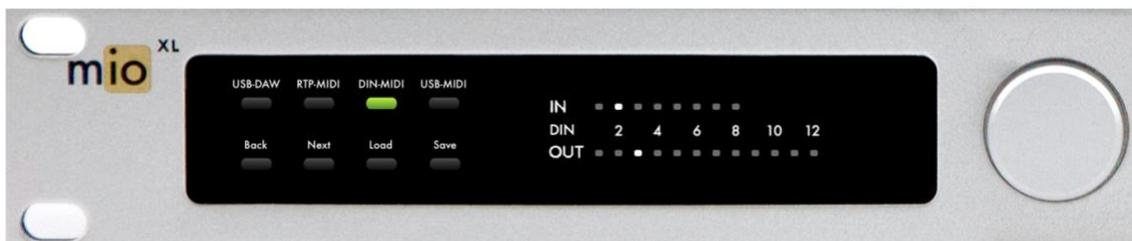
The upper line of dots indicates activity on DIN In ports 1 through 8. The lower line of dots indicates DIN Out ports 1 through 12. In this example, the two brighter dots indicate DIN-MIDI activity present on IN 2 and OUT 3.
