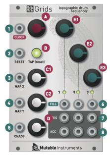
**A: Internal clock rate**. Ranges from 40 BPM to 240 BPM. When turned fully counter-clockwise, the internal clock is disabled and the unit expects a clock signal on its CLOCK input.
