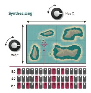
A collection of drum loops has been spatially organized and compressed into a 2-dimensional map. Using interpolation techniques, any pair of X/Y coordinates can be translated into a rhythm, with smooth morphing from one rhythm into the other.
